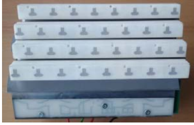
Figure 19. TX/RX 8x4 elements passive Sub-Array.
