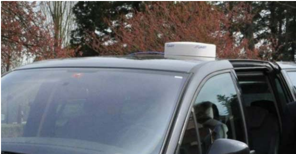
Figure 6. HiSat-30R antenna installed on car.
