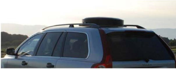
Figure 12. HiSat-60R antenna installed on car for field trials.
