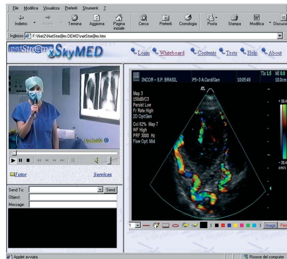
Project DELTASS: the portable terminal used by the Search & Rescue (SAR) teams to fill in the electronic patient record card. The link with the coordination centre is via the Globalstar satellite system
